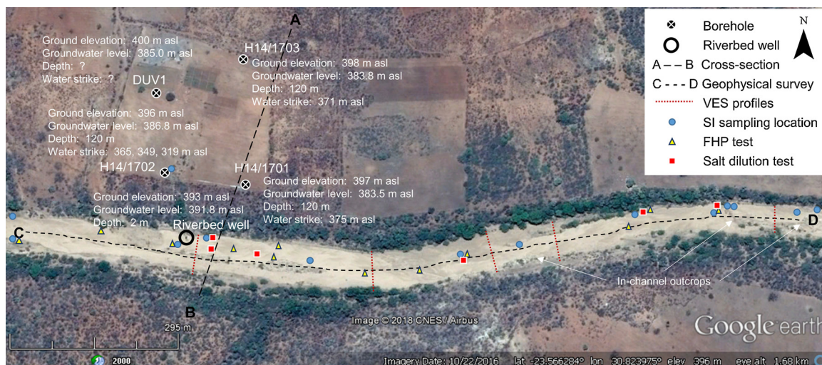
Fig. 5. Plan of the study site showing borehole information, testing and sampling locations (SI = stable isotope, FHP = falling head permeameter) and the geophysical survey lines (VES = vertical electrical sounding) along the Molototsi sand river. The elevations are taken from a 20 m DEM developed from 20 m topographic contour data and spot heights by the Department of Geography and Environmental Studies at the University of Stellenbosch (m asl = metres above sea level). Groundwater levels are as measured in October 2016. Depths and water strikes are from DWS drillers’ logs; DUV1 is an old borehole for which no logs could be found. Image source: Google earth; Imagery ©2018 DigitalGlobe.
