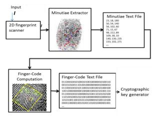
Fig. 3. Process of finger-code generation
