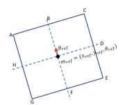
Fig. 2. A representation of a square tesselation with reference minutiae at the center.
