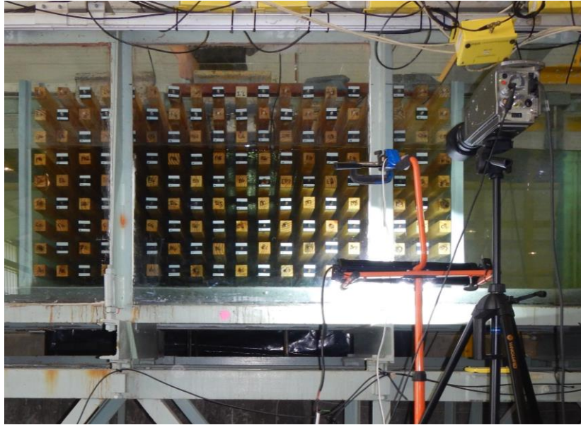
Figure 4: Image of the experimental set-up showing the high speed camera and light source.
