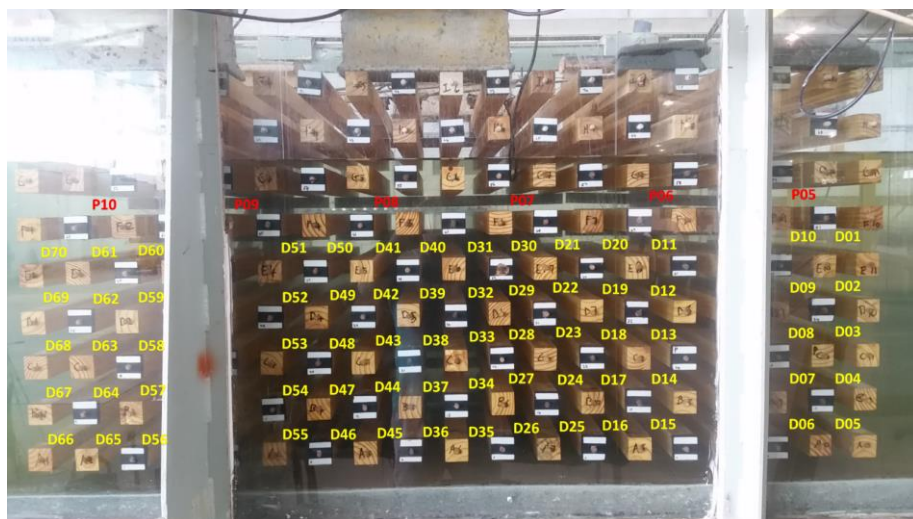
Figure 2: Ideal two-dimensional porous medium fitted in the glass flume.
