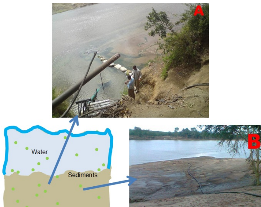
Figure 7. A scenario involving boreholes drilled inside the Limpopo river channel and contamination with cyanobacteria (green dots) cysts and akinetes for (A) irrigation farmers & (B) water utility raw water supply for human consumption.
