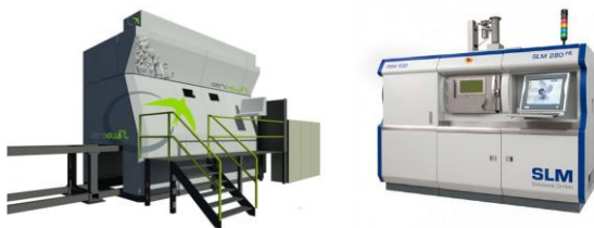
Fig. 4. (a) The Aeroswift technology and; (b) Selective laser melting system from SLM Solutions [3]
