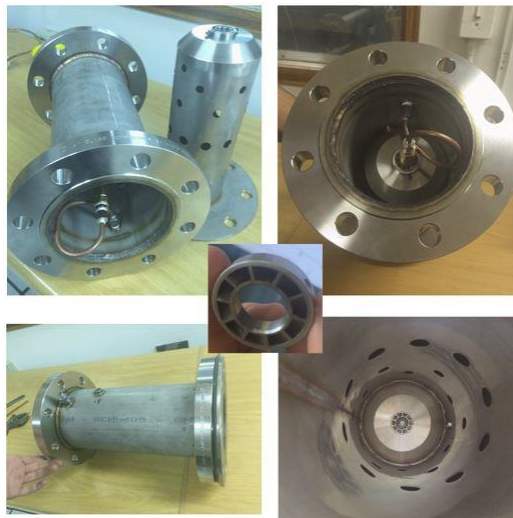
Figure 5 The manufactured combustor ready for initial testing
