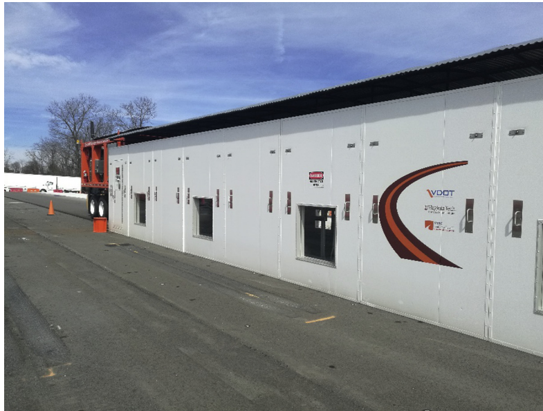
Fig. 8. HVS VI of the Virginia Department of Transportation fitted with its temperature control chamber.
