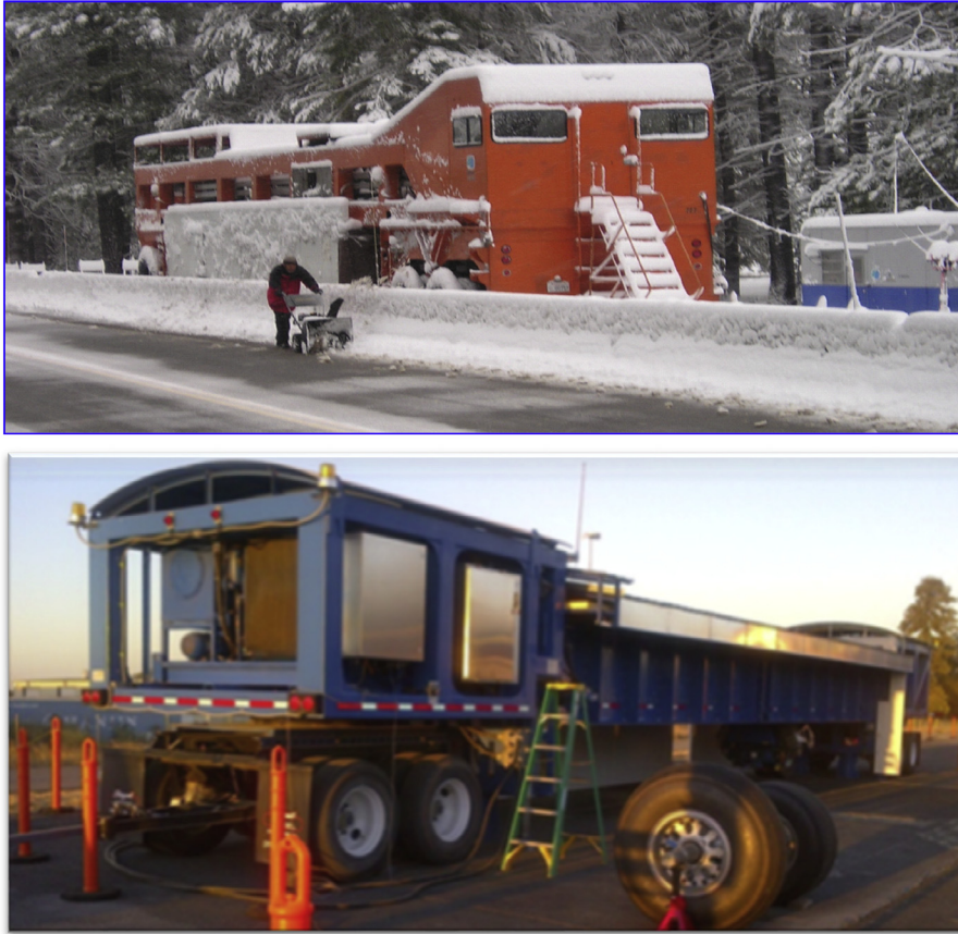
Fig. 2. The HVS Mk II and Mk VI units operational in California.
