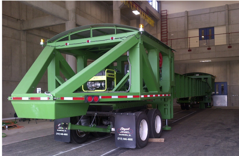
Fig. 4. The HVS Mk VI inside the testing facility of the University of Costa Rica.
