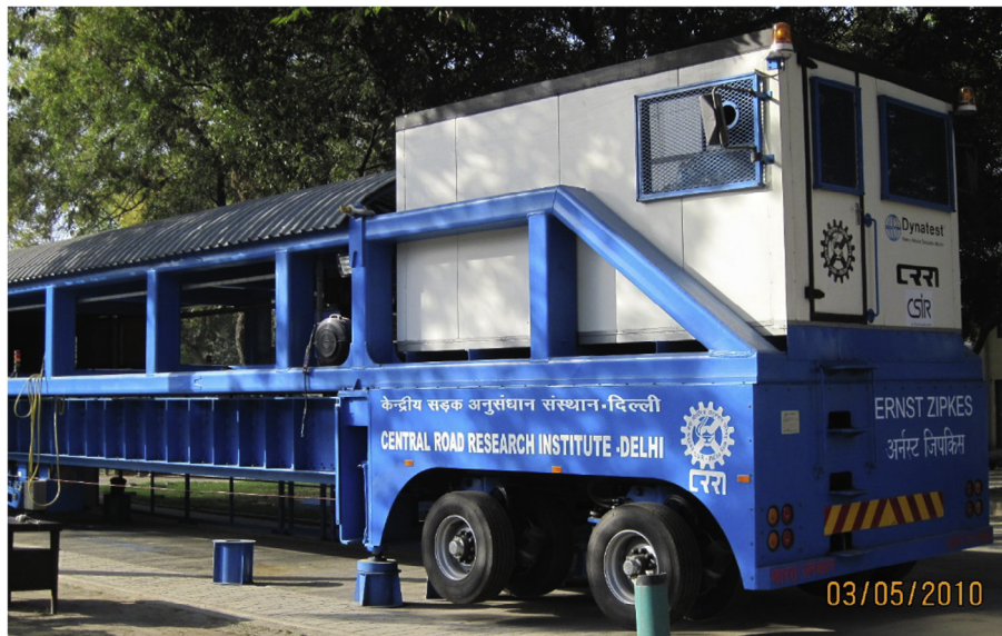
Fig. 5. The HVS Mk IV + of the Central Road Research Institute, India.
