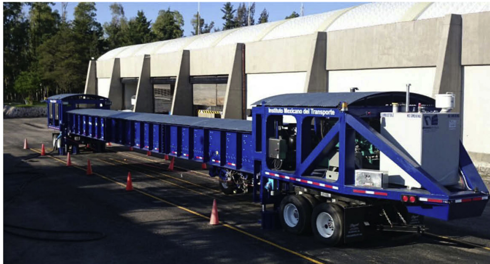
Fig. 3. The HVS Mk VI with extended beam in Mexico.
